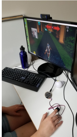
Figure 3. Game setup: Webcam, circuit playground with pulse sensor attached to finger, and game on screen.
