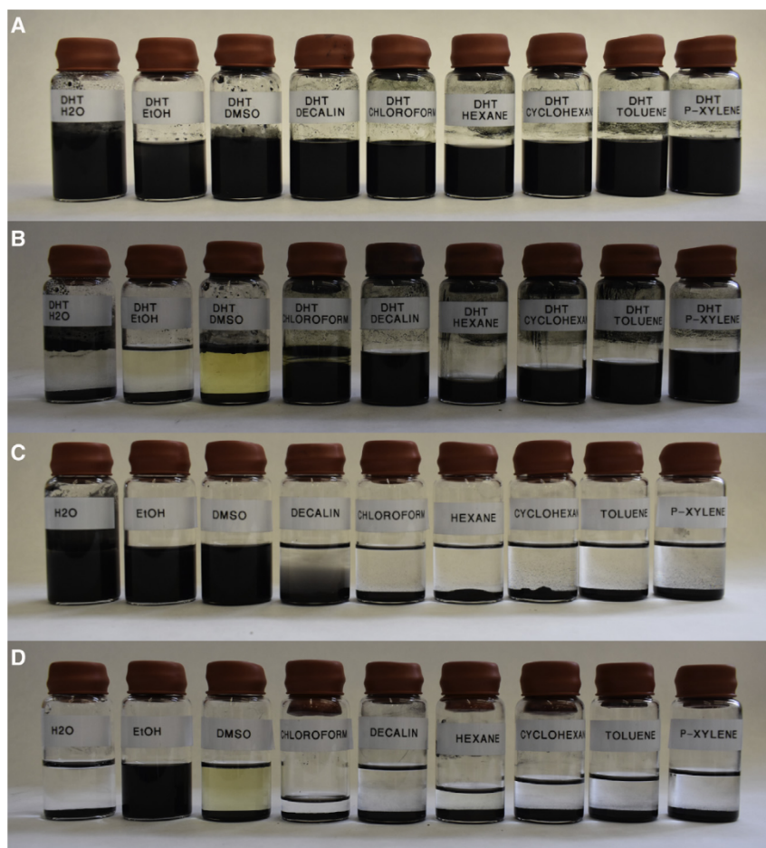
Figure 1. Photographs of \text{Ti}_3\text{C}_2\text{T}_x Suspensions in Polar (First Three Vials) and Nonpolar Solvents
