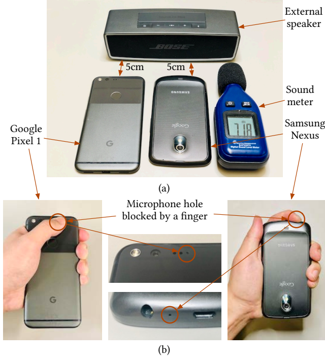
Figure 7: Experimental setup: (a) Experimental setup including smartphones used. (b) Blocking microphone holes of Google Pixel 1 and Samsung Nexus using a finger.
