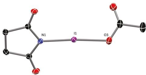
**Fig. 3** Thermal ellipsoid plot (50% ellipsoids) for the anion in  $[(C_4H_4O_2N)(OCOCH_3)](Bu_4N)$ , **12**. The cation has been omitted for clarity. Selected bond lengths (Å) and angles: N1–I1–O3, 174°; I1–O3, 2.293; I1–N1, 2.166. Tetrabutylammonium counterion is not shown for clarity.
