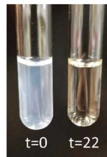
Fig. 5 Photos of Nb 94 assemblies from Fig. 4 after 0 and 22 min of irradiation.
