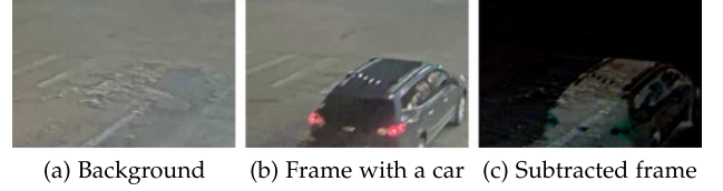
Fig. 3. An example of SDD. The subtracted frame highlights the car that entering the scene.
