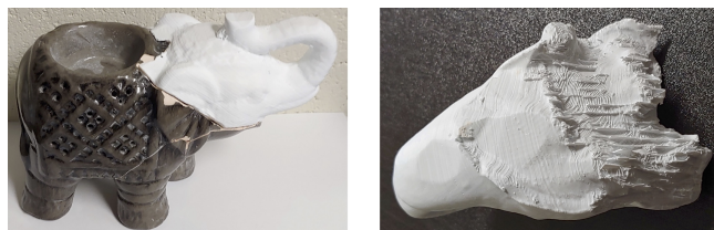
Figure 13: The 3D print of the elephant head does not make a perfect join with the elephant (left) due to uncertainties introduced by the nozzle diameter, and the presence of support structure remnants on the fracture surface (right).
