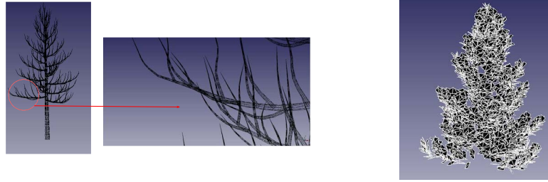
Fig. 1: Tree model visualized in a CAD viewer. (left) A 3D model of a pine tree with trunk and branches. Triangular meshes can be seen in the zoomed in view. (right) Tree is visualized with the leaves, which are modeled as triangular meshes.
