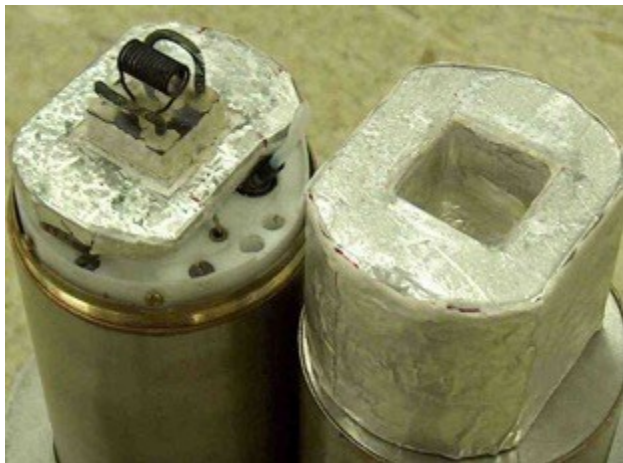
Figure 11: High temperature NMR apparatus. We fabricated this oven atop a widebore, broadband (X) probe from fumed silica tile with aluminum foil reflectors anchored by water-based cement (Omega 600 High T Cement). This apparatus can maintain sustained sample temperature up to 450^\circ\text{C} (720 K). The heating elements are spiral wound NiCr wire, which flank the tin-coated copper 13-turn NMR coil. An E-type thermocouple (Omega) sits \approx 4 mm below the NMR coil, and no forced air passes through the oven interior. We achieve typical shim-limited linewidths of 20 Hz on a 4 mm ID spherical-bulb \text{D}_2\text{O} sample. Maintaining T = 680 K ( \pm 0.2^\circ\text{C} average) requires < 8\% of the Bruker VT-3000 heater maximum power.
