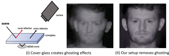
Fig. 4: The coverglass induces ghosting and double images. With a combination of using Brewster’s angle, NIR notch filter and absorbing baffles, we eliminate the ghosting.
