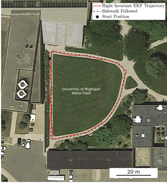
Fig. 11. Long outdoor odometry experiment where Cassie walked roughly 200 m along a sidewalk over 7 minutes and 45 seconds. A video of this experiment can be found at https://youtu.be/jRUltB_dMlo
