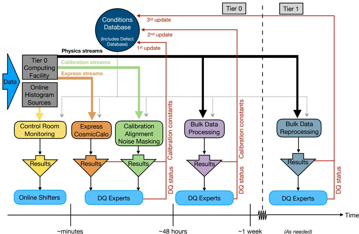
**Figure 2.** Schematic diagram illustrating the nominal Run 2 operations workflow for the data quality assessment of ATLAS data. Online histogram sources include the high-level trigger farm, the data acquisition system, and full reconstruction of a fraction of events accepted by the trigger.
