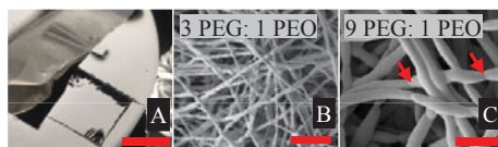
Figure 3. A The fiber blends shown were ES onto RTDs so that change in resistance under light illumination could be measured. When PEG-only was ES, the deposited material was paste-like. (Scale = 1cm) B-C SEMs showing PEG/PEO polymer blend ES into fibers. Increased PEG in the fibers resulted in weaker fibers which were pulled apart at various locations throughout the fibers (examples indicated by arrows). (Scale = 5 \mu m)
