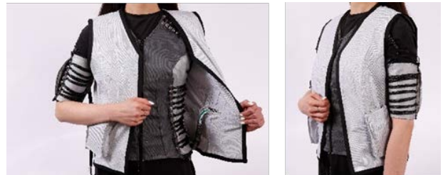
Figure 1: Final garment design (Gen. 3) with SMA actuators
