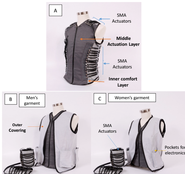
Figure 6: (A) Inner comfort layer and middle actuation layers with integrated SMA actuators on the torso and
