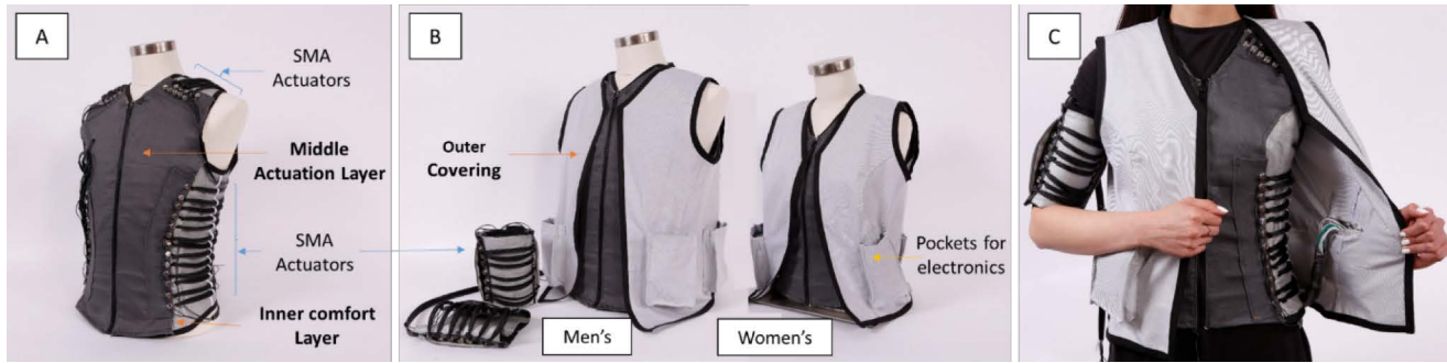
Figure 1: System components and design. (A) Comfort layer and actuation layers with SMA actuators on torso / shoulders; (B) Final garments with outer covering and arm bands; (C) Women's garment showing all components (layers
