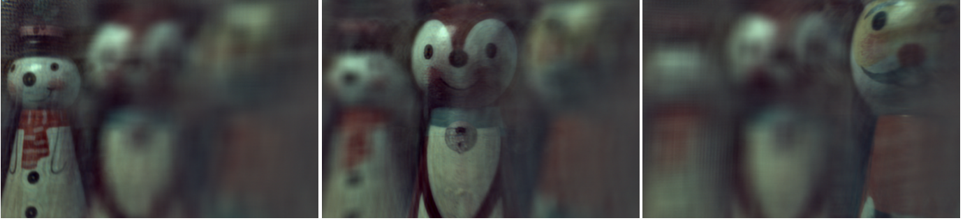
Fig. 1. Lensless focal stack . We show images reconstructed at three different depths using our proposed SweepCam technique, which is a lensless camera with a programmable mask.
