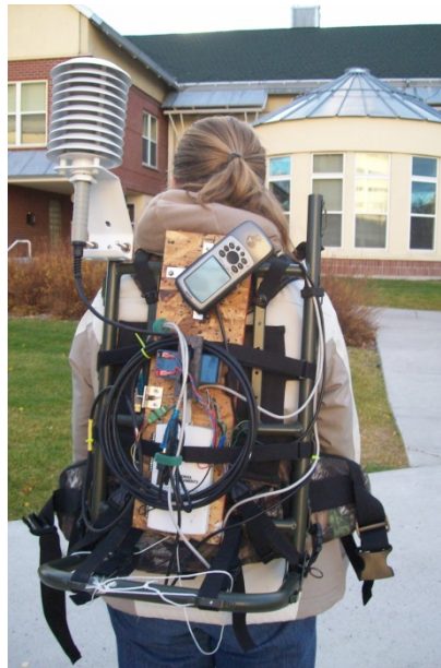
Figure 2. Mobile backpack-mounted weather station with GPS for mapping meteorological data.
