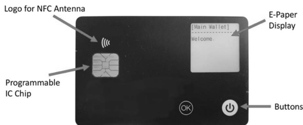
Fig. 3. Smart card with an e-paper display, physical buttons, and a programmable IC chip
