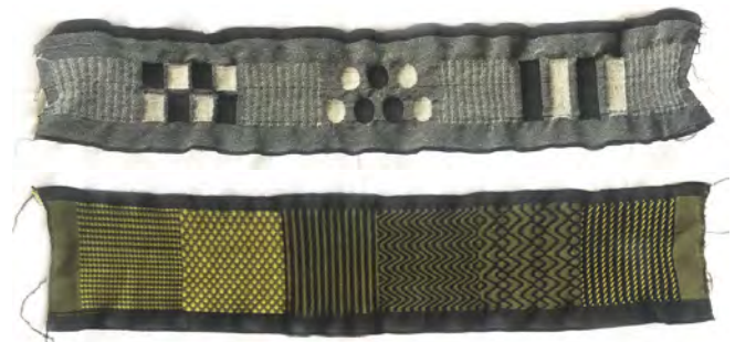
Figure 4. Test swatches exploring (top) various shapes of stuffed pockets and their integration within elastic structures and (bottom) several stitches to test in terms of the flexibility they provide to the overall weave.
