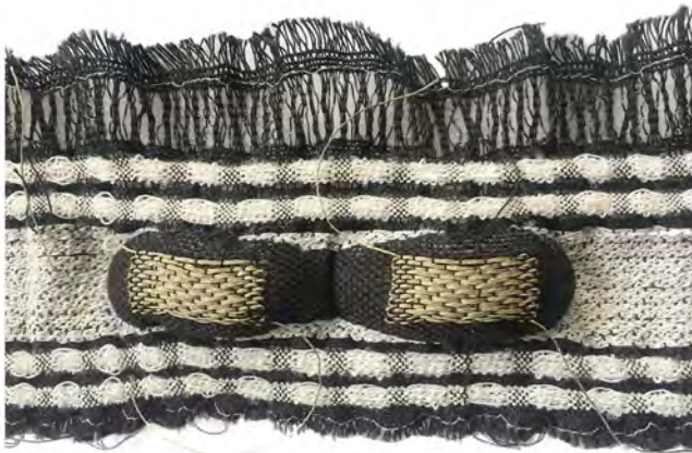
Figure 3. The design challenge that Katya and Sandra focused on was weaving head-worn electrodes for sensing muscle stimulation in the forehead. This image shows a detail how silver threads were integrated in conjunction with elastics, wool, and cotton to rest comfortably and firmly on the forehead.
