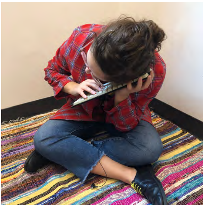
Figure 4. The listening jacket turns on live binaural audio feedback when a hand cups the ear. In this example, the gesture is being used to augment the sound of a discarded computer keyboard. Several methods were developed and tested for the cupping gesture and the styling reflects the designers personal tastes.
