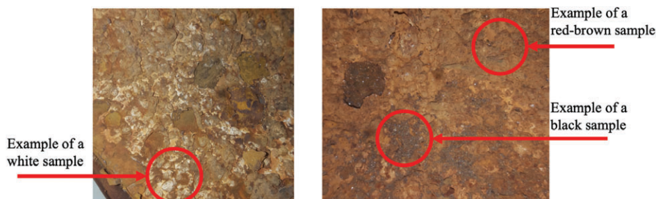
FIGURE 2 Pipe inner-wall samples collected post-Sn addition showing all three different collected samples: red–brown, white, and black.
