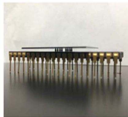
Fig. 11 Assembled and packaged SolarPede die carrying a payload
