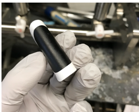
Figure 7. Demonstration showing that due to the use of a cross-linking agent, the membrane can be rolled or bent multiple times without developing any cracks.
