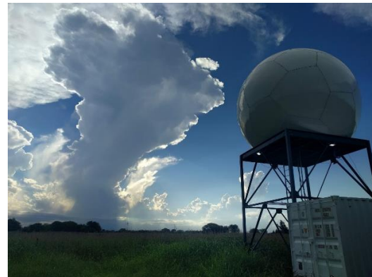
Figure 2. CSU C-Band radar deployed near Alta Gracia – Argentina during RELAMPAGO
