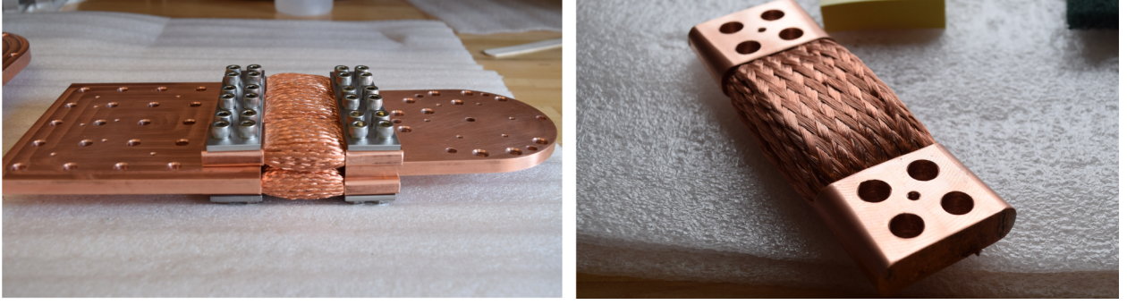
Figure 5: Left: A completed heat strap composed of 6 braid assemblies. A thin stainless steel plate distributes the force of the bolts and nuts across the surface of the braid ends. Right: A single 7-layer braided strap. This strap is created by inserting layers of OFHC braid into a short OFHC tube and compressing under 20 tons of pressure in a hydraulic press.
