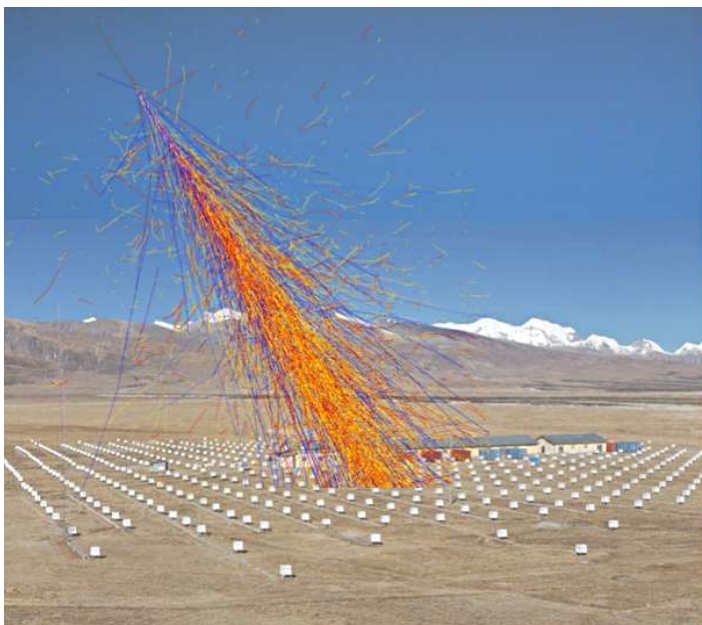
Figure 1: The Tibet AB \gamma experiment is located at an altitude of 4300 m in Yangbajing, China. With an array of scintillation detectors and underwater water-Cherenkov detectors covering 65,700 m 2 , the experiment measures the secondary particles that are produced when a high-energy photon strikes the upper atmosphere. An artist's depiction of such an air shower is shown in the image. (Tibet AS \gamma Collaboration)
