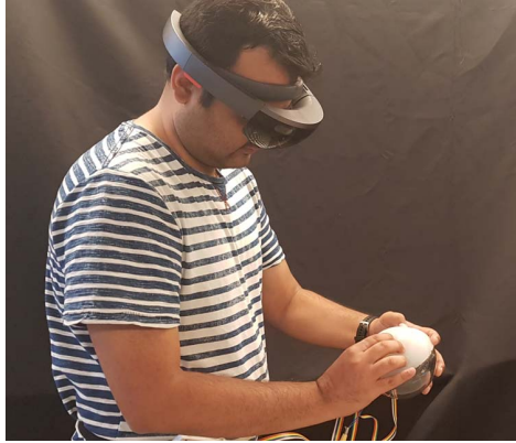
Figure 12: A user interacting with Squishy Device and viewing the manipulation of the virtual object in Microsoft Hololens.
