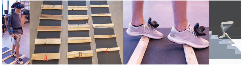
Figure 1: (Left) A user ascending virtual stairs on prototype. (Middle Left) Physical prototype. A-Elongated ramp. B-Elongated ramp with a bump. C-Normal ramp. (Middle Right) A user's feet on ramps, descending virtual stairs. (Right) Virtual stairs and legs in a VE.
