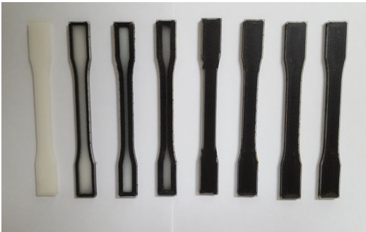
Figure 4 Tensile specimens printed with Markforged: (left to right) Nylon, CF2RC, CF4RC, CF5RC, CF0RI, CF2RI, CF4RI, CF5RI (see online version for colours)
