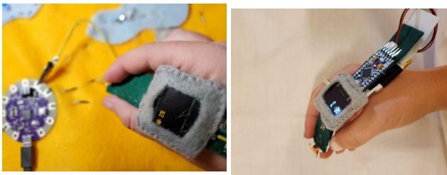
Figure 1: The "low-Floor" multimeter measures voltage and continuity in an E-textile circuit.
