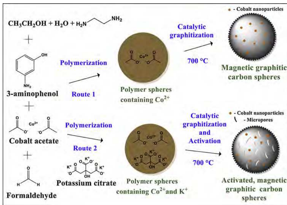
Scheme 1. Synthesis routes to obtain magnetic graphitic carbon spheres (route 1) and activated magnetic graphitic carbon spheres (route 2).
