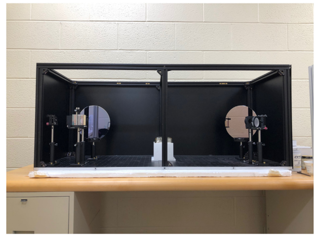
Fig. 22. Picture of optics setup in black-anodized light tight box.
