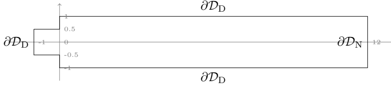
FIG. 6.1. Symmetric step domain with boundary conditions.
