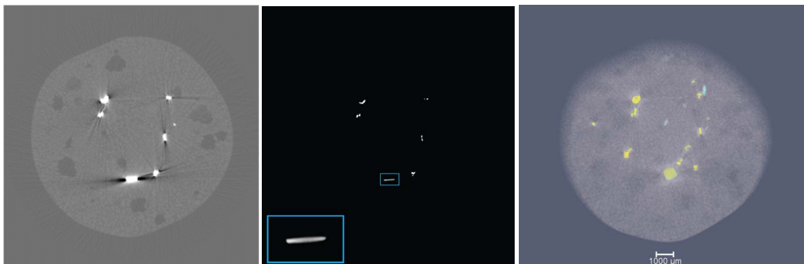
Figure 1. (left) Example CT image of artificial quartz + epoxy core with embedded gold and iron particles. Gold grains are accompanied by moderate to severe streaking artifacts. (center) Re-windowed version of left image, showing gold grains closer to true dimensions. Overall variations in brightness are due to variable degrees of blurring based on particle size and shape, though the flat grain in bottom center and enlarged in inset has a dimmer center and brighter ends due to beam hardening. (right) 3D rendering of core. Quartz is semi-transparent white, gold particles are yellow, iron shavings are light blue, and air bubbles in epoxy appear as darker regions.
