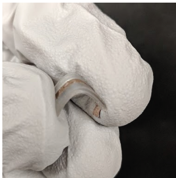
Figure S20. Image of a bent solid-contact reference electrode.
