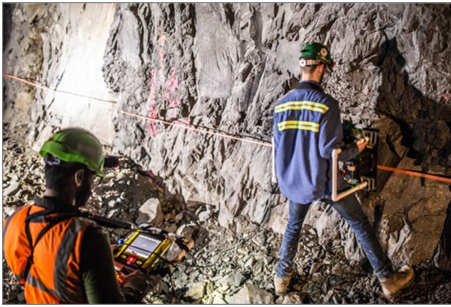
Fig. 8 The 200-MHz survey in progress
