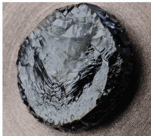
FIG. 1. Photograph of the 2 mm thick ScN layer on a 9 mm diameter W (100) substrate.
