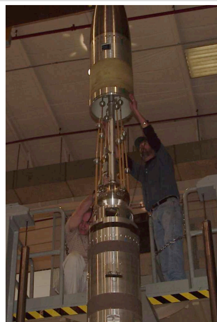
Figure 5. Electric field probes as deployed in sounding rocket 21.116.
