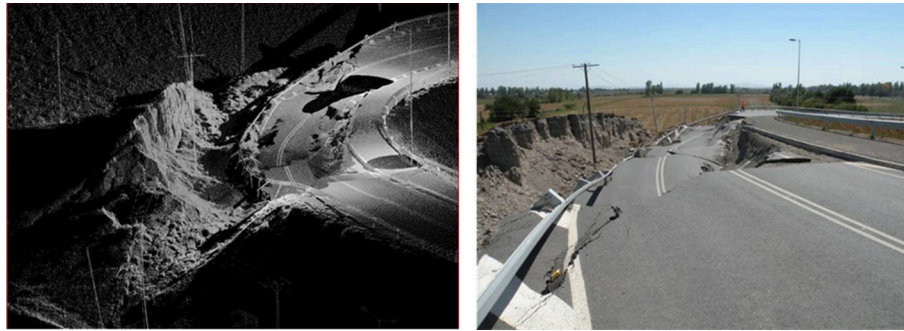
FIGURE 4 | Ground-based LIDAR and optical images of a failed overpass embankment on Ruta 5 as a result of the 2010 Chile Earthquake (LIDAR survey by Kayen presented in Bray and Frost, 2010).
