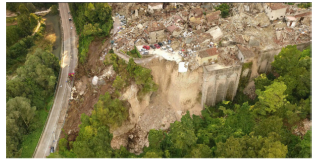
FIGURE 7 | 3D SfM model of a slope failure in Pescara del Tronto possibly caused by a retaining wall collapse (N42.75109°E13.27208 °; SfM by Franke et al. presented in Zimmaro and Stewart, 2016).
