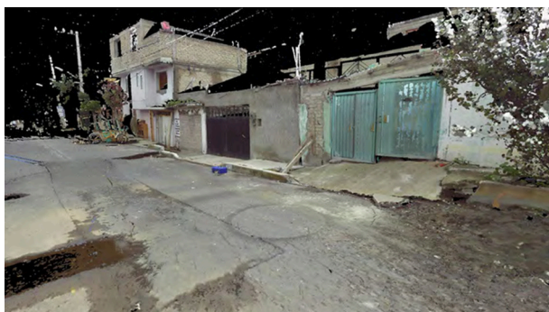
FIGURE 11 | LIDAR model showing ground failure in Colonia del Mar (N19.2851°, W99.0579°; Mayoral et al., 2018).
