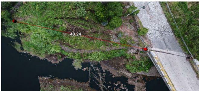
Figure 9. 3D model of a landslide adjacent to the Rio Yautepec Bridge created using SfM from UAV images (N18.7306°, W99.1194°; Mayoral et al. 2018).
