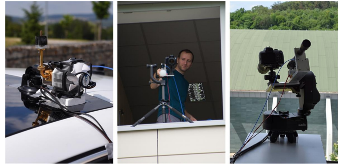
Fig. 5. From left to right: placement of TX antenna on the car roof, RX antenna on the gimbal head and on the motorized mount.
