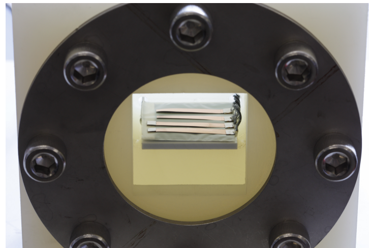
FIGURE 4. TRANSPARENT BATTERY PROTOTYPE: ELECTRODE SETUP IN TEST CHAMBER BEFORE DRYING
