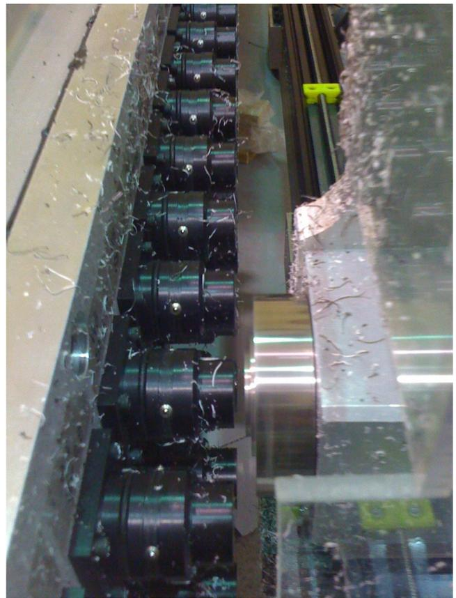
Fig. 15. Fly cutter of fiber cutting machine making an initial milling pass of PCAL WLS fiber bundles.
