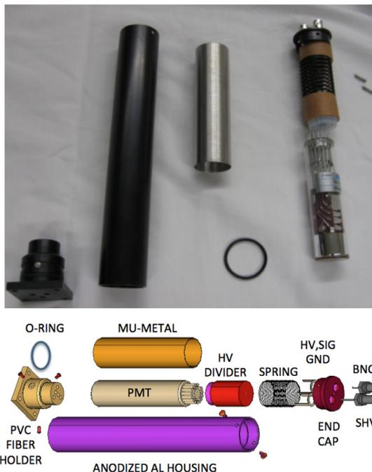
Fig. 10. Photograph and schematic shows the housing assembly for the Hamamatsu R6095 1-in diameter PMT used in PCAL. The bulkhead mount fiber holder was outfitted with an O-Ring and three push-fit ball plungers to ensure a snug and light-tight push-on fit for the PMT housing.
