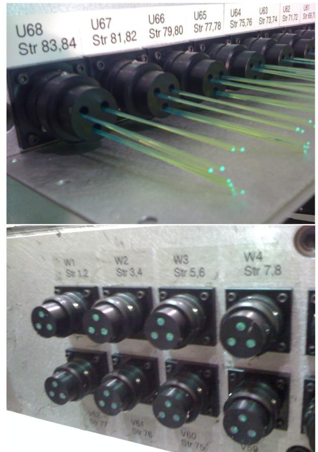
Fig. 8. Top: WLS fibers from the scintillators extending from the PMT attachment mounts fixed to the PCAL bulkhead. Bottom: WLS fibers after gluing, milling, and polishing prior to PMT installation.
