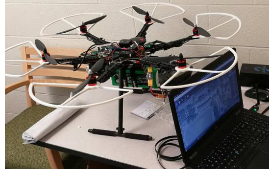
Fig. 3. Prototype of the UAV-based Air Monitoring System
