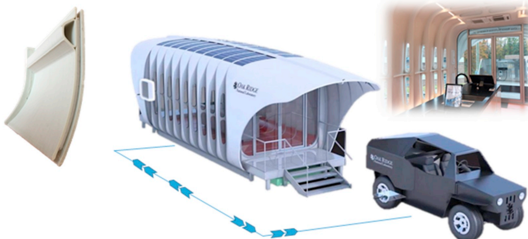
Fig. 4. 3-D printed vehicle by the ORNL, which remotely connects to a 3-D printed house (photo courtesy: Dr. Som Shrestha, Oak Ridge National Laboratory).
