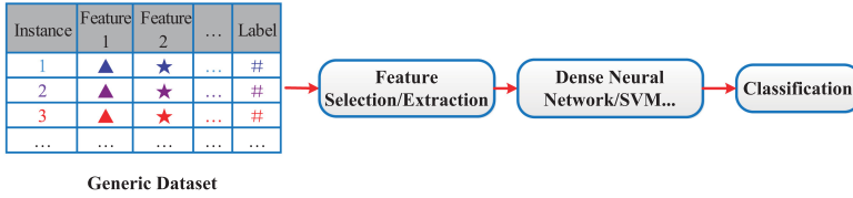
Fig. 2. Typical workflow of applying traditional machine learning methods to generic data for classification tasks, where generic data is shown in the form of instance-feature table and instances are assumed identical and independently distributed (i.i.d.).
