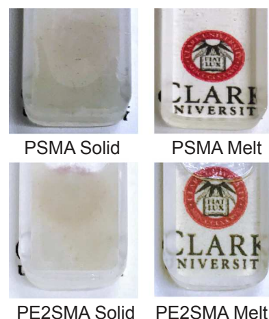
Fig. 6. Opaque and transparent phases of PSMA (top) and PE2SMA (bottom).
