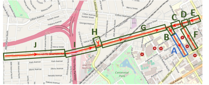
Fig. 12: Road segment for congestion event 10 in Table I. The source road of congestion is road segment 'A'. Following the congestion at the source road segment, the congestion propagates to the 1st ('B', 'C', 'G') and 3rd hop ('D', 'E', 'F', 'H', 'I', 'J') incoming neighbors respectively.
