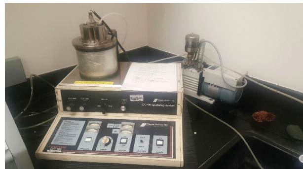
Fig. 6 CrC 100 sputtering system used for coating the nonconductive samples with silver
