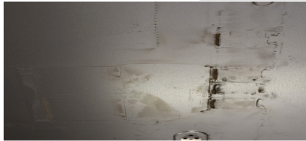
Fig. 3 Lodged dust at the different locations of the test server
