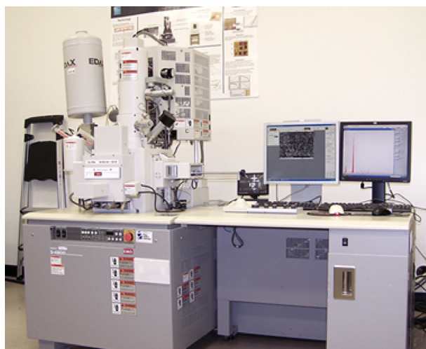
Fig. 5 Hitachi S-4800 II FE SEM with cold field emission source
