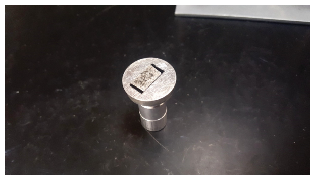
Fig. 7 Sample holder with the silver-coated sample
