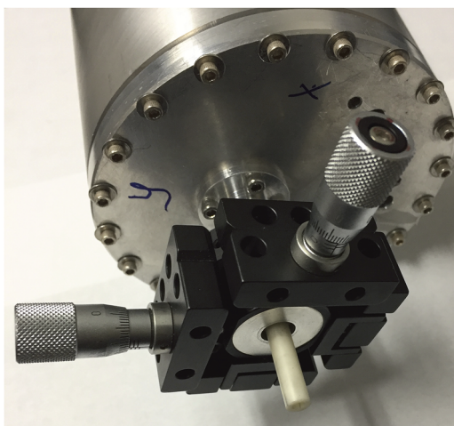
FIG. 5. Micrometer system used to control tilt of the rod. The tight collar is not shown in this photo.
